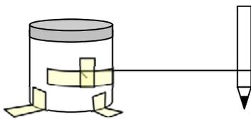
Tie one end of the string to the pencil. Use the sticky tape to fix the other end to the side of the upturned glass.
